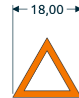
DETAIL A | TACTILE WARNING SCALE 1 : 1
