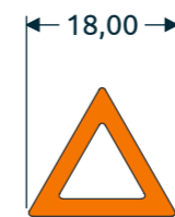
DETAIL A | TACTILE WARNING SCALE 1:1
