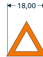
DETAIL C | TACTILE WARNING SCALE 1 : 1
